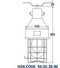
SUPPLY OF FLAMEPROOF/EXPLOSION PROOF WELL GLASS LIGHT FITTING WITHOUT CONTROL GEAR. CONSTRUCTED FROM DIE CAST ALUMINIUM ALLOY LM-6, SUITABLE FOR INSTALLATION IN GROUP IIA, IIB GAS AREA SUITABLE UPTO 60 W INCANDESCENT LAMP OR UPTO 16W CFL LAMP BUT WITHOUT BULB, SEPARATE TERMINAL CHAMBER AT THE TOP FOR EASE OF MAINTENANCE. LOOP IN LOOP OUT CAN BE DONE. BOROSIL GLASS WITH WIRE GUARD AND J HOOK ARE PROVIDED. TYPE: HY62,
